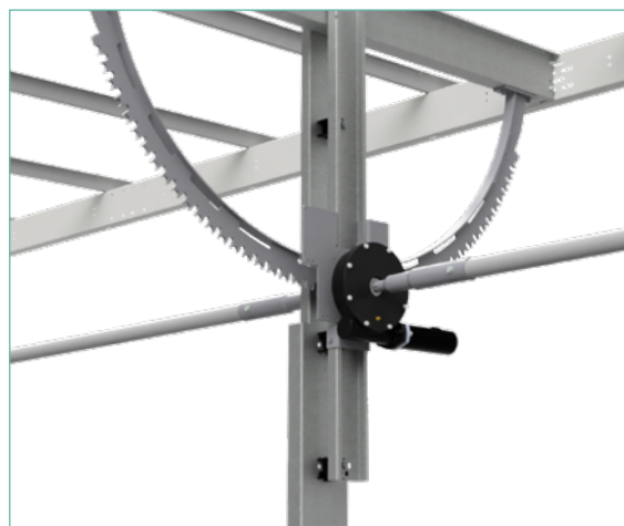
Girder assembly with drive and control unit
